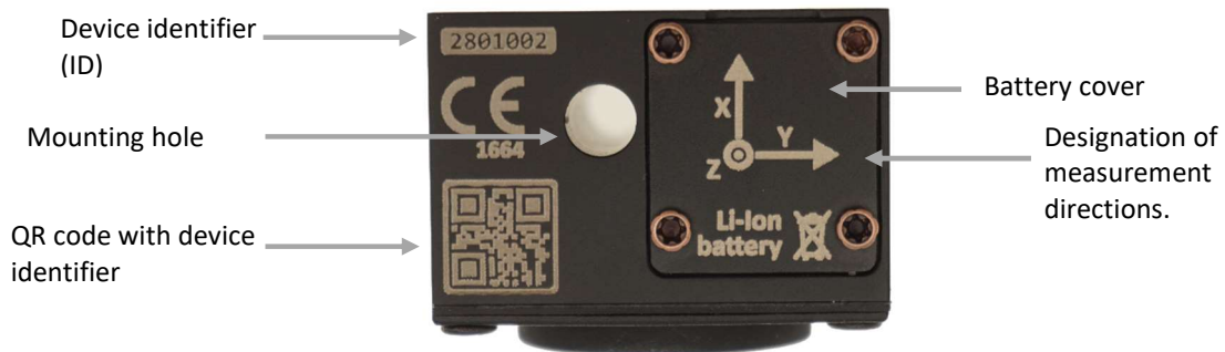
Fig. 2. View of the upper part of the device housing
