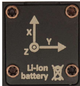
Fig. 19. Designation of vibration measurement directions
