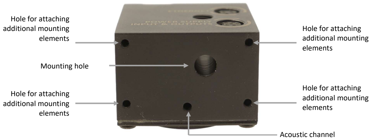
Fig. 6. View of the underside of the device
