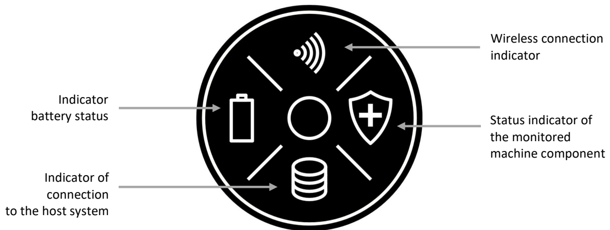
Fig. 7. View of CL@VE sensor keypad
