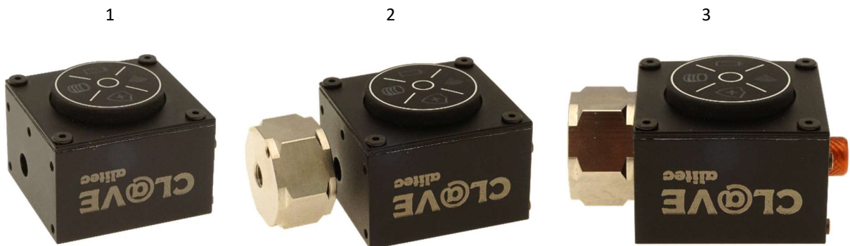
Fig. 16. Attaching a magnet holder to the sensor
