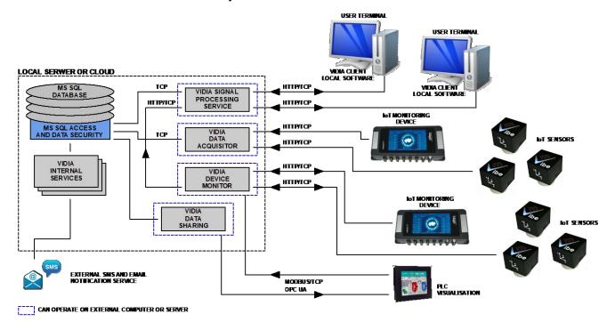
Versatile solutions allow a high level of customization in the field of implementation hardware and communication channels. The highest level communication protocol is based on the HTTP/HTTPS standard. It allows to send control frames as well as raw vibration and process signal data. The chosen services communicate with database using MS SQL secured connection. The database and specified services can be hosted on separate server if needed.
